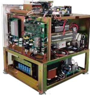
32kW / 40kW Super Capacitor Bank (PSU Generator)
